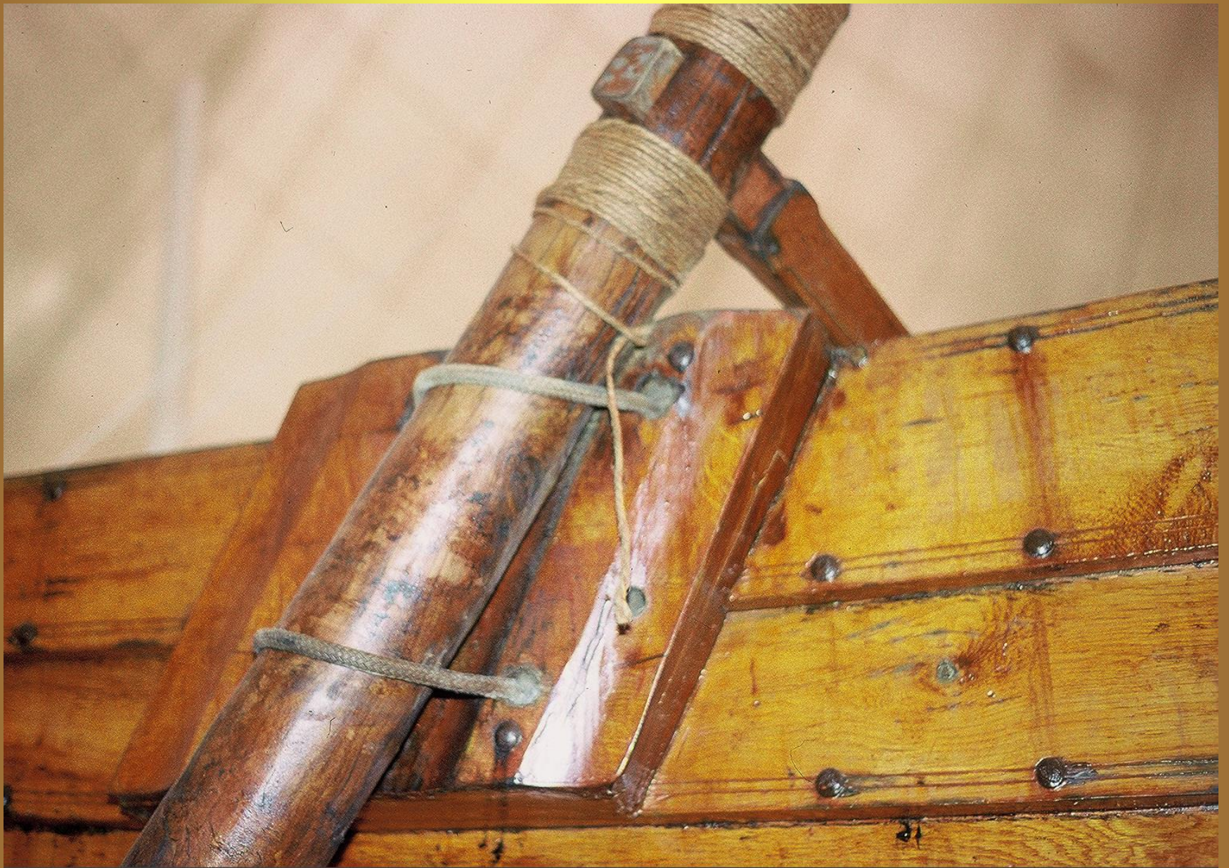
Rudder connected gunnel with ropes.
