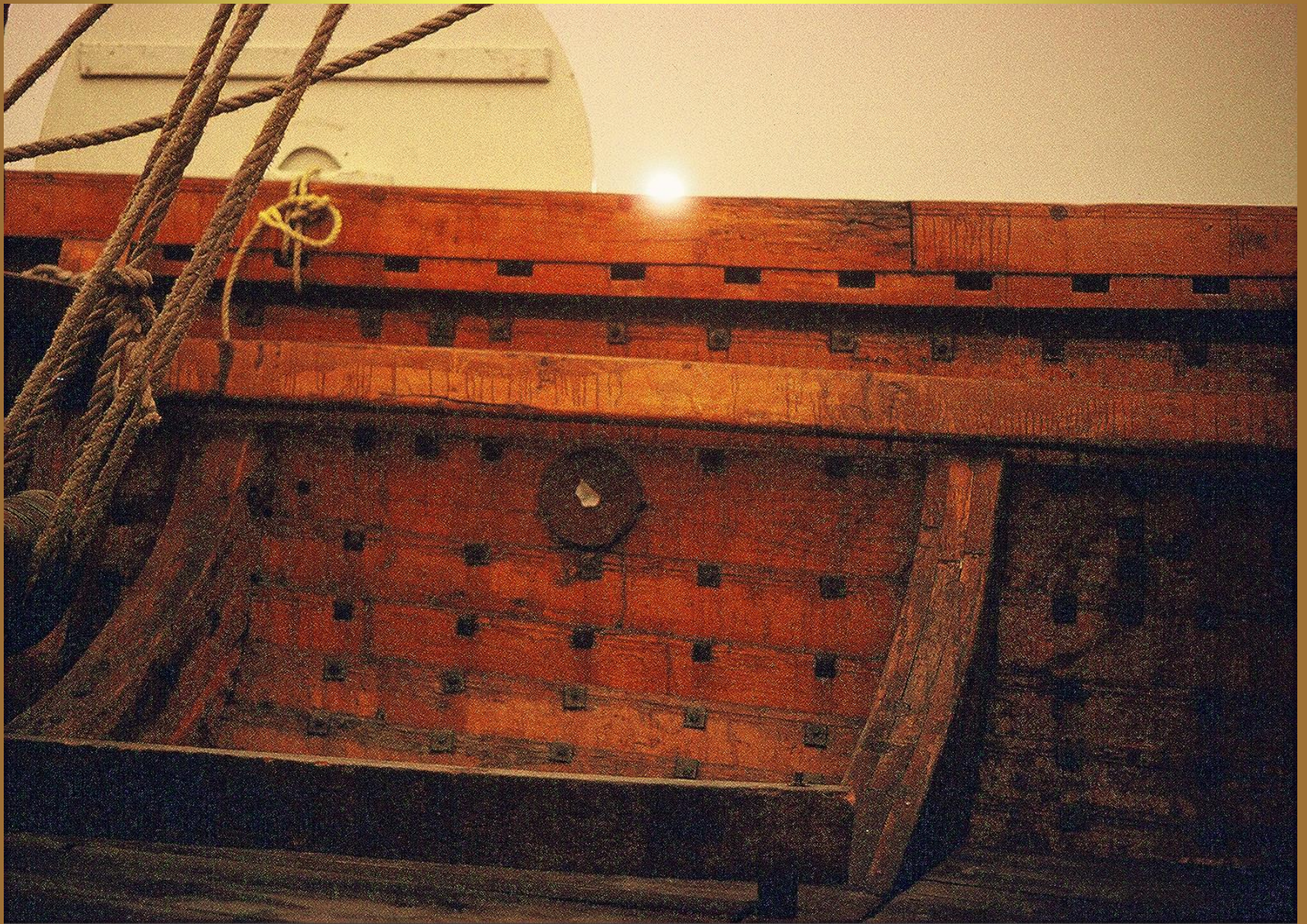
Inside showing the planking held together by iron rivets.
